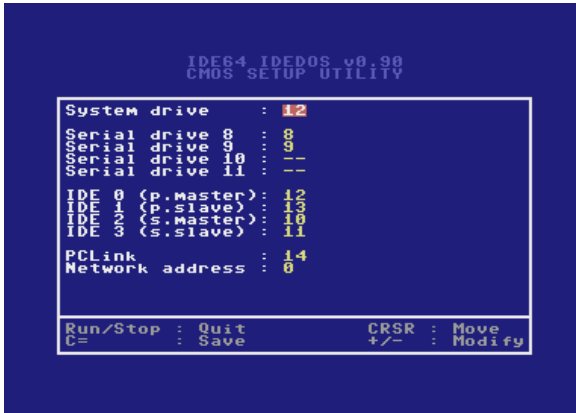
Figure 4: Device number setup screen of the setup utility
